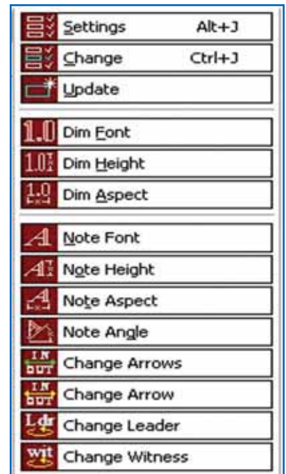
Figure 5. The Detail Settings dialog box lets users choose a range of settings such as dimension fonts, note fonts, leader types and arrow styles.
